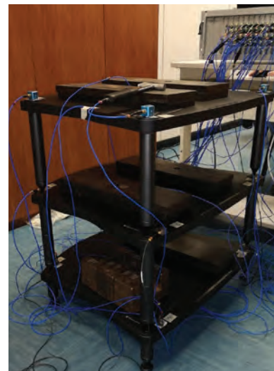
Loaded rack during modal tests.
