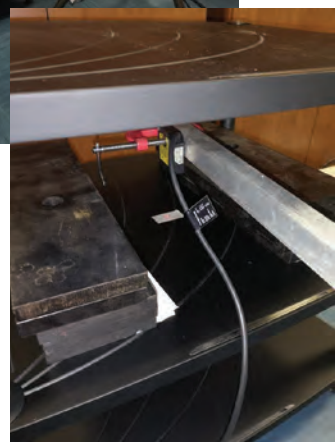
Rack during static tests: middle shelf loading.
