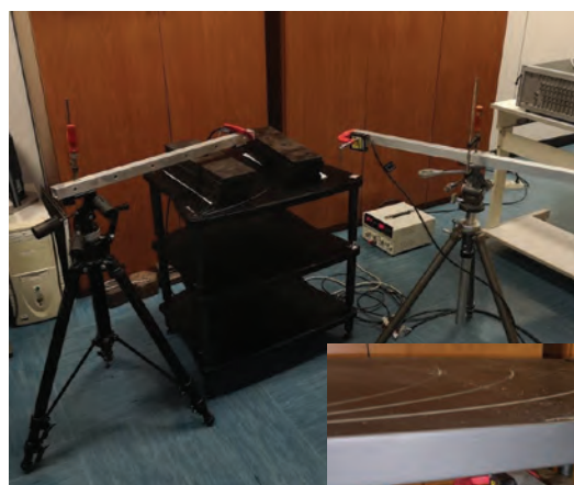
Rack during static tests: top shelf loading.
